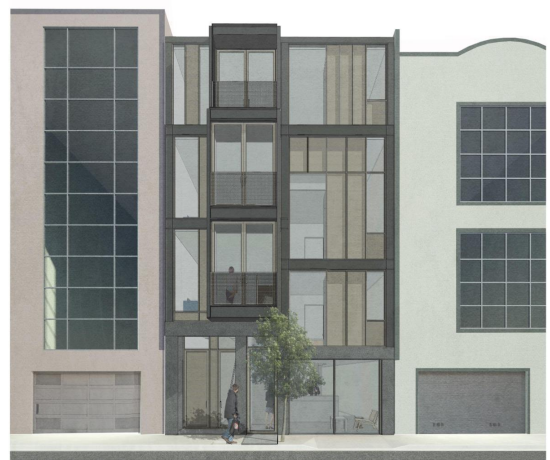
option a1 - concrete framed base / black steel frame w/ bronze aluminum (brighter/lighter) framing & infill panels
