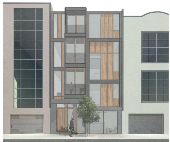
option b - concrete framed base / black steel frame w/ timber infill framing & panels
